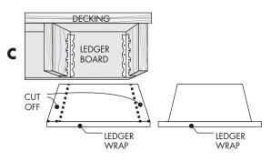
Slide the Ledger Wrap up between the joists and fasten at the top edge using 1-1/4" galvanized or color-matched exterior trim nails. Nail the Ledger Wrap flanges into the bottom of the joists using color-matched exterior trim nails. (see illus D)
