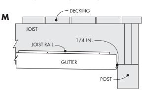
**If you DO use rain gutters**, measure the full joist length and cut the Joist and Boundary Gutters 1-3/4" shorter than that measurement to allow for drainage. (see Illus. N)
