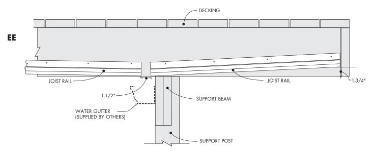
On the cantilever end only, apply a 4-6" weatherproofing tape over the joist rails, its fasteners and the joist. Then apply a bead of exterior grade caulking at the top edge of the weatherproofing tape to ensure a good seal. Measure, cut and fasten a Water Diverter onto the deck rim joist. (see Illus. FF). Refer to Step 1 on page 2, to install the Water Diverter.
