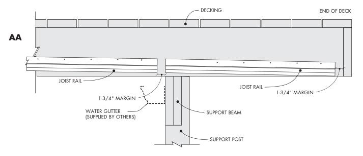
Install an 18" wide piece of weatherproof tape over the joist rails, its fasteners, and onto the joist, keeping an equal amount of tape on both sides of the support beam as shown below. Add a bead of exterior caulking on the top edge of the tape to ensure a good seal. (see Illus BB)
