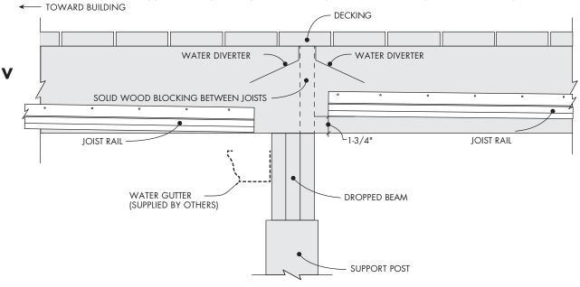
Measure, cut and install Joist/Boundary Gutters. NOTE: Before installing the Gutter, adhere the Foam Seal and apply a bead of exterior caulk to the Gutter as shown in Step 7 on page 6 where illustrated below. (see Illus. Z).
