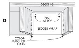
Continue adding Ledger Wrap between subsequent joists following the previous instructions. The Ledger Wrap flanges will overlap.
