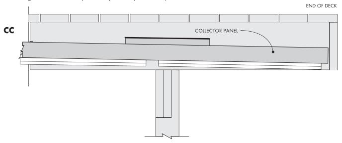
Measure, cut and install the Joist/Boundary Gutters on the cantilever end. Allow a 1/4" margin at the end of the joist for expansion. The notched area of the Gutter above the support beam is not required, but creates a nicer visual. Hint: Use a scrap piece of Joist Gutter to create a template for the notch. NOTE: Before installing the Gutter, adhere the Foam Seal and apply a bead of exterior caulk to the Gutter as shown in Step 7 on page 6 where illustrated below. (see Illus. DD).
